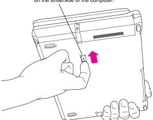
To unlock the module, slide the latch on the underside of the computer.
